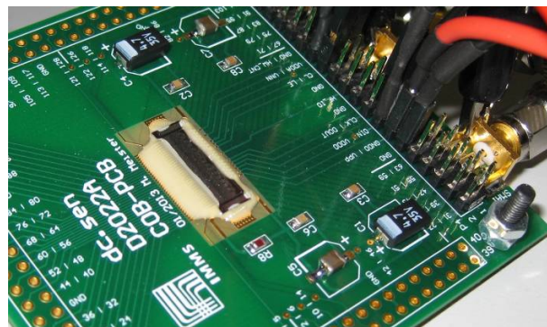
Fig. 1.: Multiplexer on evaluationboard for characterization
