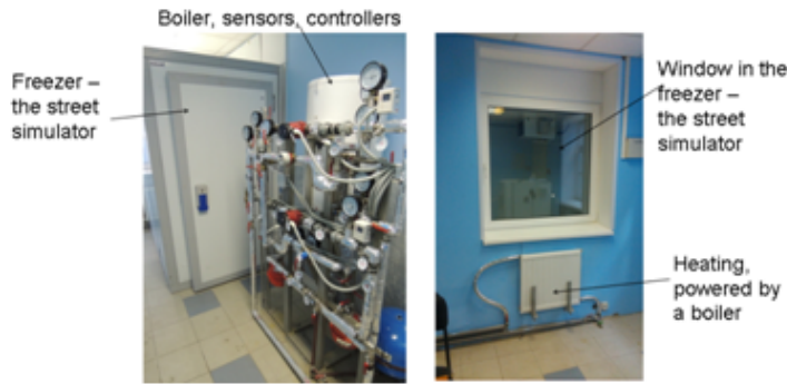
Fig. 2. Laboratory of the ITMO University "Sensors and Sensor Networks in Energy Saving"
