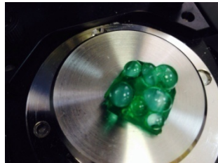
Fig. 1: Hydrogel with sorption of ions of copper on the ATR prefix.
